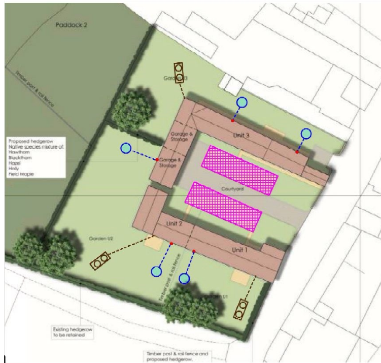
Fig 2: Outline Drainage Strategy, with SuDS permeable paving identified by the pink hatch.
